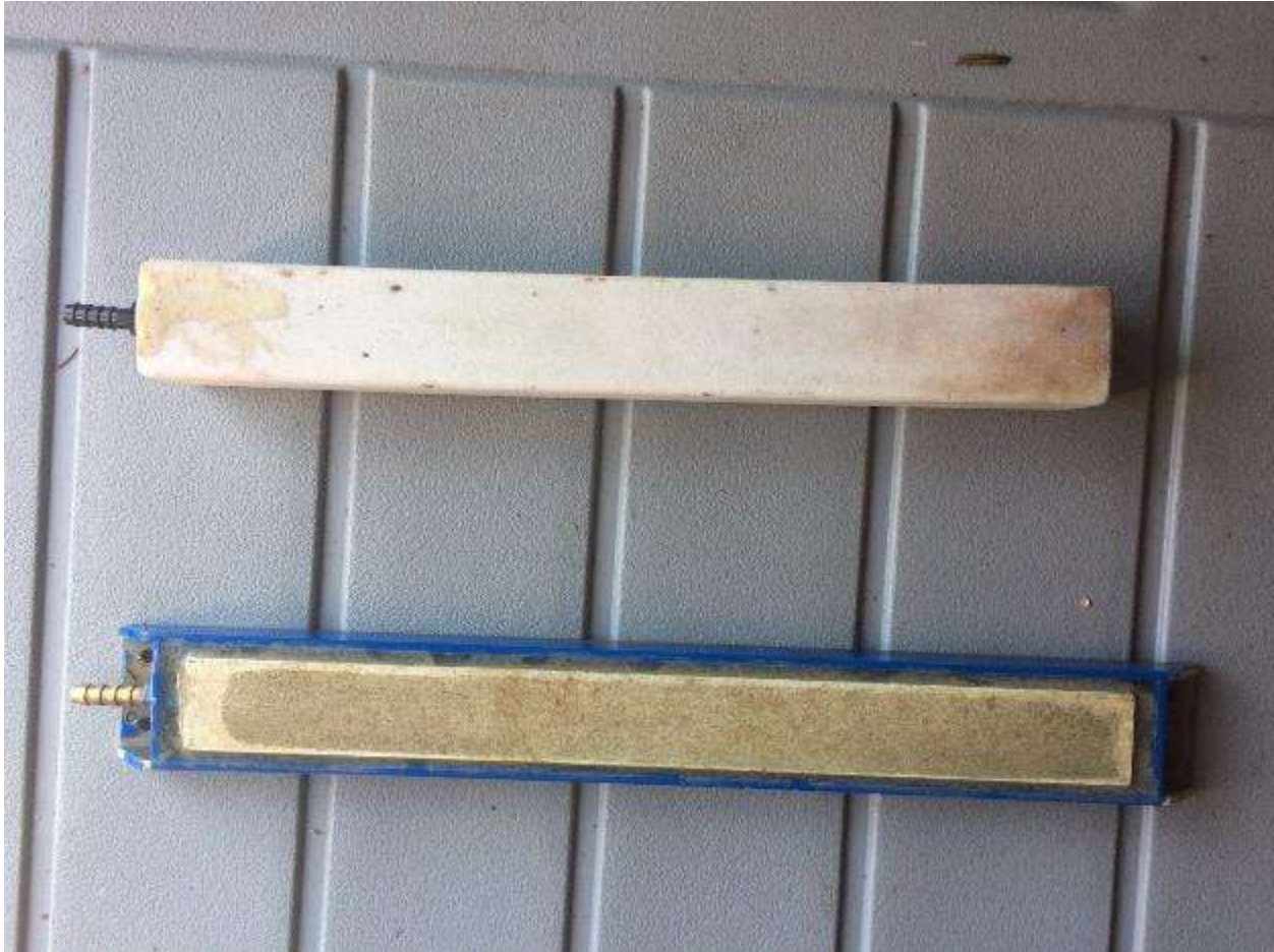
Figure 3.1-6: Air and Oxygen Diffusers for the Conowingo Eel Collection Facility Tanks, 2017
